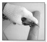
Place your finger between the buckle ears. Tighten band clamp by turning the tension handle clockwise.
