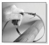
Insert the band into the buckle. The buckle teeth shall be in the direction of the operator with the ears faced up. Bend end of band under buckle.
