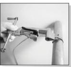
Place band in opening of tool nose and gripper Block. Push the "tool nose" against the buckle
