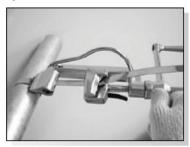
When reaching the desired tension, turn the tool over the buckle. This movement will increase the band tension.
