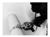
**3.** Hold short handle in right hand. Push long handle forward in full arc with left hand. This tightens the band.
