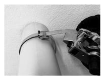
**1.** Insert the band into the buckle. The buckle teeth shall be in the direction of the operator with the ears faced up. Bend end of band under buckle.
