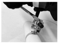
**4.** When reaching the desired tension, turn the tool over the buckle. This movement will increase the band tension.
