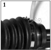
Wrap the clamp around the CV boot and thread the tail through the buckle. Draw it tight.
