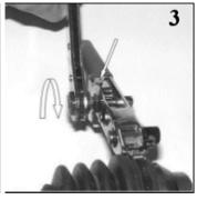
Depress the locking pawl and tension the clamp with a clockwise motion of the ratchet.
