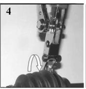
After sufficient tension has been applied (the clamp is tight enough to hold the boot from turning on the joint but not too tight that the boot is damaged), lever the tool back over the buckle to put a bend in the clamp to hold the tension.
