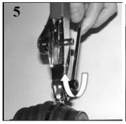
Cut off excess band with the cutter and remove the tool.
