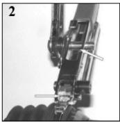
Insert the tail of the clamp into the head of the banding tool and slide it through the slot of the winding mandrel.
