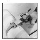
Press the tensioning handle several times until the buckle is tight.
